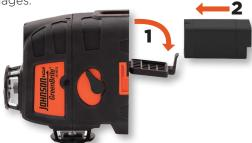
To use 4 x AA Alkaline batteries: Insert the batteries into the battery holder according to the indicated polarity, lift the latch on the battery door and insert the battery holder into the laser. Press the battery door closed until the latch engages.
